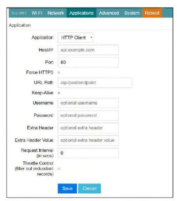
HTTP connections. When the interval is set as 0, the data will be sent immediately. When it
