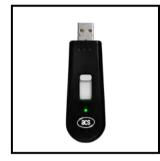
The ACR1251T is the token version of the ACR1251U PC-linked NFC smart card reader, which was developed based on the 13.56 MHz contactless technology. Following the ACR122T, the token version of the ACR122U, the world's first CCID-compliant contactless reader, the ACR1251T offers more and advanced features. It is designed to support not only ISO 14443 Type A and B cards, but also MIFARE®, FeliCa and all four types of NFC tags and devices.
