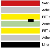
Satin Adhesive PET substrate layer Antenna PET substrate layer Adhesive Liner
