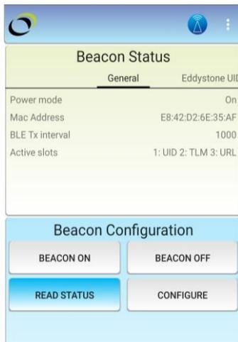
After successfully scanning a Confidex Viking™ beacon, the tabs in the **Beacon Status** window show the general settings as well as settings for each active configured slot. Different tabs can be accessed by swiping horizontally. Status information is displayed in the app until another beacon is scanned, or the app is restarted.
