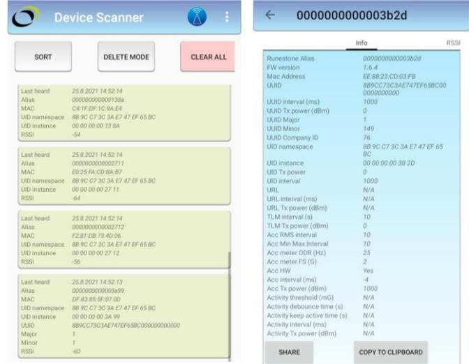
Device scanner shows the latest RSSI (Received Signal Strength Indication) value and timestamp from the last received packet. Device list can be sorted or cleared with the buttons on top of the list. **Device details** view can be opened by pressing a beacon on the list.
