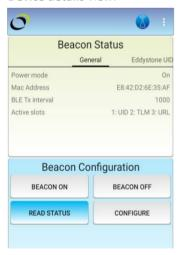
After successfully scanning a Confidex Viking<sup>TM</sup> beacon, the tabs in the **Beacon Status** window show the general settings as well as settings for each active configured slot. Different tabs can be accessed by swiping horizontally. Status information is displayed in the app until another beacon is scanned, or the app is restarted.
